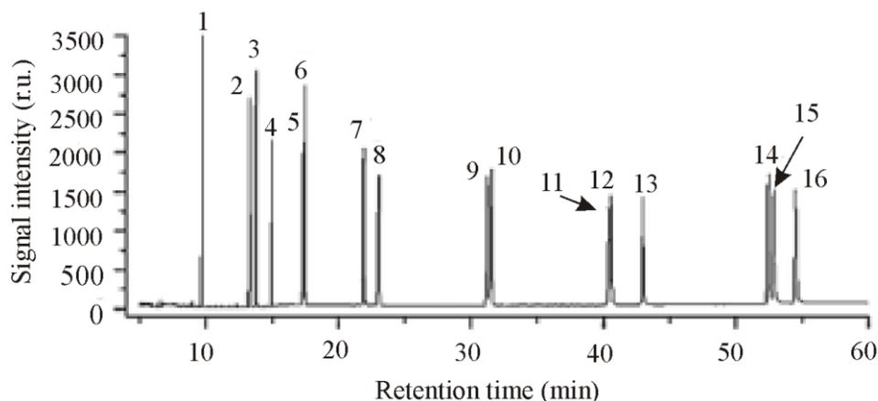
Figure 1. GC-MS chromatogram of a standard mixture of the sixteen EPA-PAHs.
